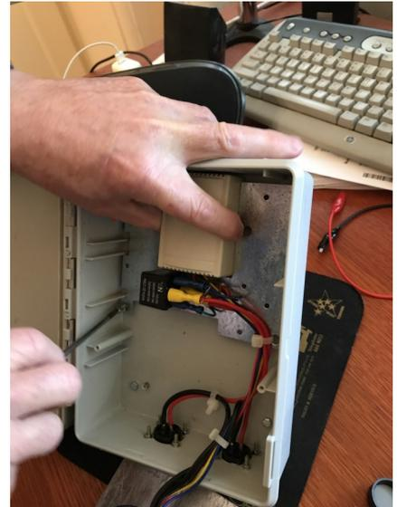
3. Push transceiver box out of mounting plate.
