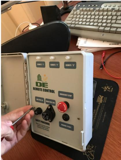
1. Remove two screws on faceplate to remove front panel.
