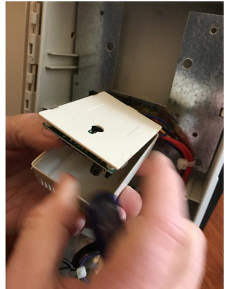
6. Press red button inside receiver box while pressing button on remote transceiver fob red light will flash.
