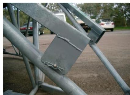
will now lower the field bin front to the ground when filling and The “Easy hitch” can be left in this position while travelling (make sure the bolts are not too tight as this will restrict movement).
