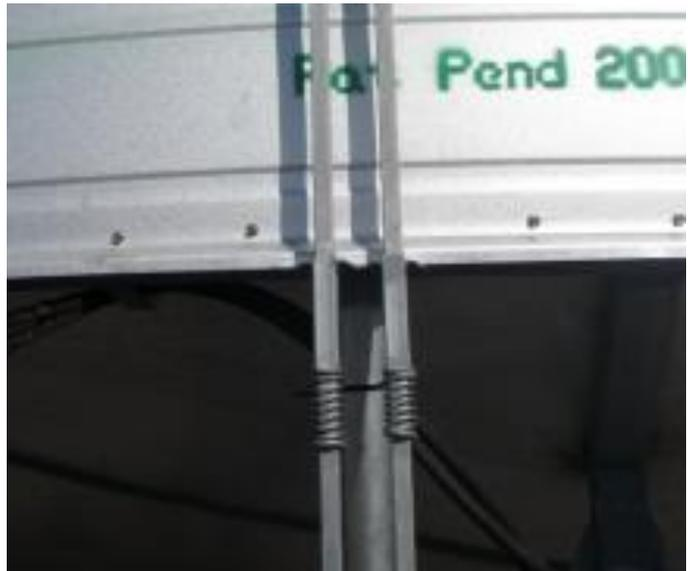
4.2 Pull the square tube above the spring downwards to release the handles and always open the top panel first, then secure lifting again to prevent wind damage.
