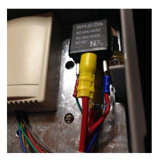
If clutch drops in and out while energised the 12 volt relay may need replacing.
