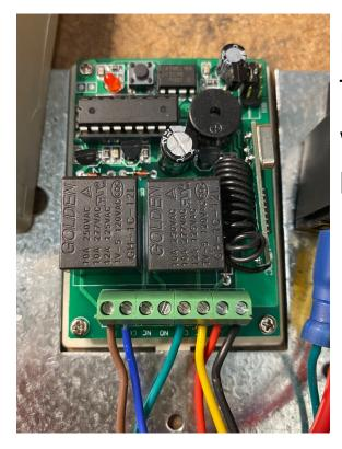
If remote unit is not working: Take out 6 coloured receiver wires, replace unit and re-wire as before or as per this picture.
