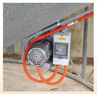
DE Engineers manufacture our own aeration fans and unique louvered ducting to push cool dry air to the bottom of silos to ensure all the stored grain is kept in optimum condition. NB/-sealed grain storage allows moist air into silos damaging grain and rusting silo walls.
